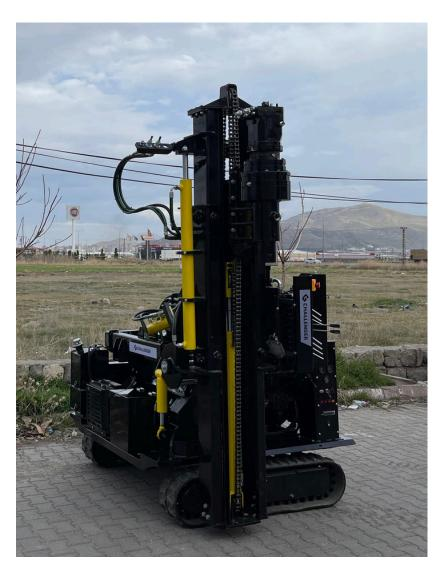
The Quantum SD Series is a versatile and highefficiency machine designed for demanding construction and infrastructure projects. Engineered specifically for driving and fastening ground screws, it ensures quick and reliable performance with simple, single-operator functionality. Available in two models, the 600 SD and 800 SD, the series offers robust design and precision to meet diverse project needs.
