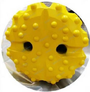
The **QUANTUM** DTH Hammers are designed to optimize the use of compressed air flow and incorporate the most efficient materials for each component. They are capable of drilling through compacted soil, rock, and concrete. Hole diameters can be customized **between 2 inches and 10 inches**, with shaft lengths available up to **3 meters**.
