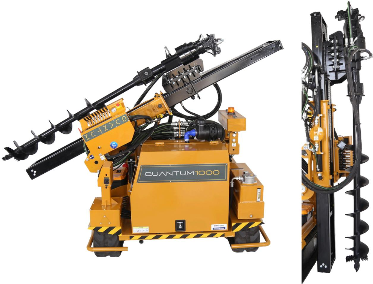
**Quantum** Hydraulic Earth Auger is a highly efficient tool designed for excavation in various terrains and soil types. The auger operates both clockwise and counterclockwise. Hole diameters can be customized **between 100 mm and 450 mm**, while the shaft length can be produced up to **3 meters**.
